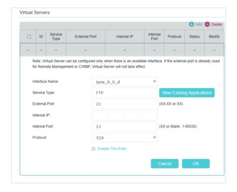
5. Enter the IP address of the computer running the service application in the Internal IP field.
