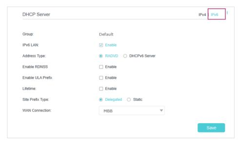
1) Select RADVD as the address type to make the router assign IPv6 address prefixes to hosts.
