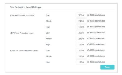
2. The protection will be triggered immediately when the number of packets exceeds the preset threshold value, and the vicious host will be displayed in the Blocked DoS Host List.
