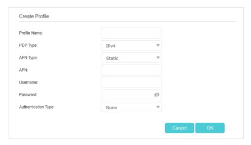
5. Click OK to make the settings effective and the new profile will be used to set up a new connection.
