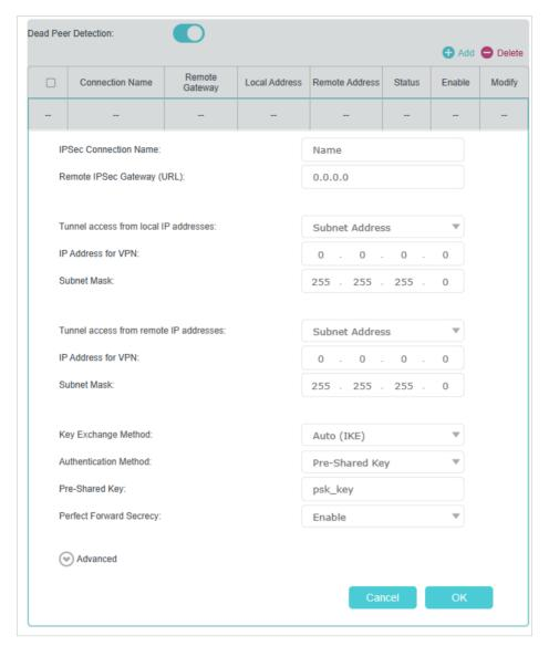
5. Configure the advanced settings according to the following explanation. We recommend that you keep the default settings. If you want to change these settings, make sure that both VPN server endpoints use the same Encryption Algorithm, Integrity Algorithm, Diffie-Hellman Group and Key Lifetime in both phase1 and phase2.
