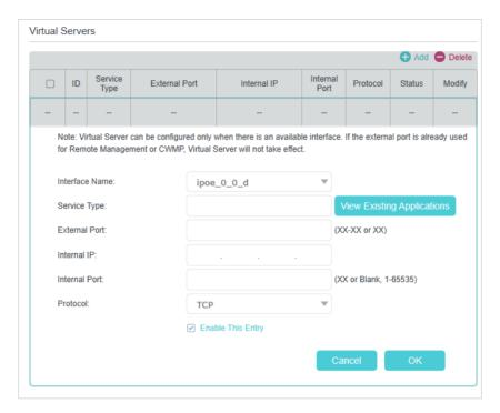
4. Click View Existing Applications to select a service from the list to automatically populate the appropriate port number in the External Port and Internal Port fields. If the service is not listed, enter the External Port number (e.g. 21) or a range of ports (e.g. 21-25). Leave the Internal Port blank if it is the same as the External Port or enter a specific port number (e.g. 21) if the External Port is a single port. The following picture takes application FTP as an example.
