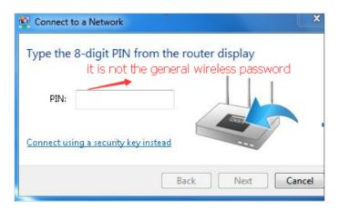
If you cannot find the PIN or PIN failed, you may choose Connecting using a security key instead, and then type in the Wireless Password/Network Security Key. 3) If it continues to show note of Network Security Key Mismatch, it is suggested to confirm the wireless password of your wireless router.
