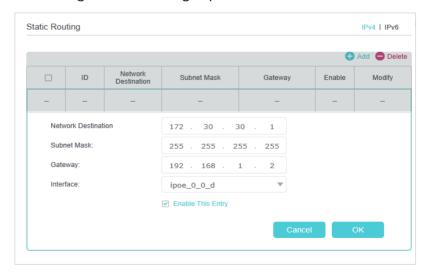
Network Destination: The destination IP address that you want to assign to a static route. This IP address cannot be on the same subnet with the WAN IP or LAN IP of the Router A. In the example, the IP address of the company network is the destination IP address, so here we enter 172.30.30.1.
