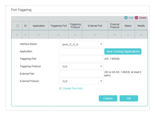
3. Click View Existing Applications, and select the desired application. The Triggering Port, Triggering Protocol and External Port will be automatically filled in. The following picture takes application MSN Gaming Zone as an example.
